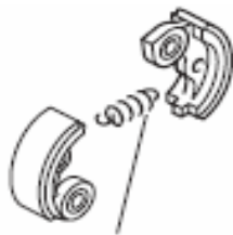
Tension spring 6 (231858-8) Free length: 27 mm
