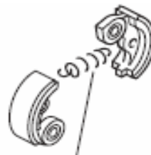
Tension spring 7 (231881-3) Free length: 35 mm
